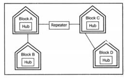
For Layout 1, since the cabling distance between Blocks A and C, and that between B and C are quite large, so a repeater each, would ideally be needed along their path to avoid loss of signals during the course of data flow in these routes.
